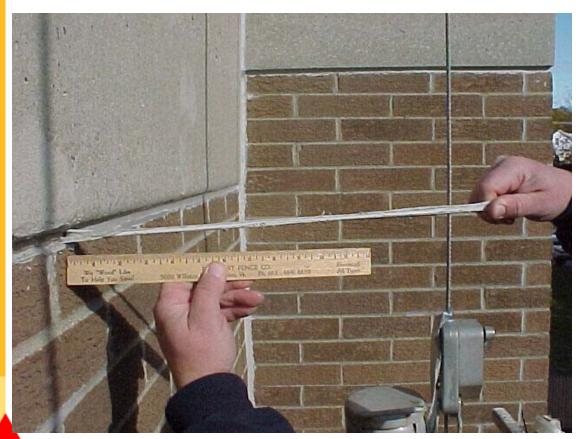
Place sealant and allow to cure. Cut a 2-3" piece of the sealant and pull at a 90° angle from the substrate. The sealant should not "peel" from the joint interface.
