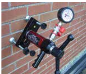
Mortar Joint Performance Test
