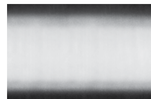
Latex paint through a HEA 517 tip at 1,000 PSI
