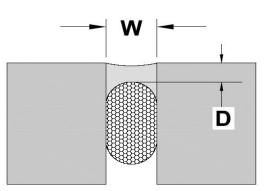
EXPANSION JOINTS - The minimum width and depth of any sealant application should be 1/4" by 1/4" (6 mm by 6 mm). The depth (D) of sealant
