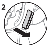
Gun unlocked (gun will spray)
